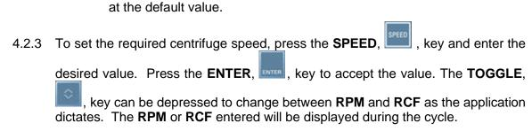
Note: The minimum centrifuge speed is 300 RPM and will auto correct to this value if one is entered below this value.
