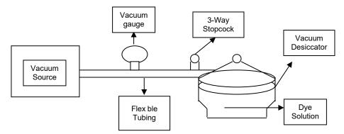
5.2.2 Make sure the vacuum source is able to provide at least 25" Mercury vacuum.
