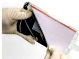
Fig. 3 Removing laminated sealing from Anode (bottom) stack
