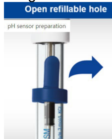
Image 4: Ensure Filling Hole is Secured
