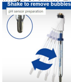
Image 5: Shake Electrode While Holding Top to Remove Bubbles
